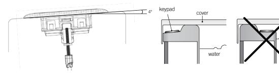
When installing the keypad on the spa, a minimum angle of 4 degrees must be respected.
